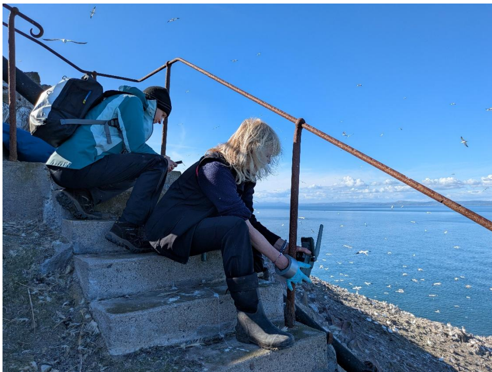
Figure 2. Installation of Trail Cam 2, situated on a railing beside the steps leading down to the foghorn, with the square solar panel visible on top of the camera beside the aerial. This location was in shade for at least half of the day. Photo credit © SSC.
